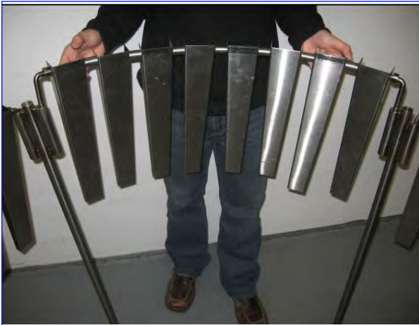
Photo 5 Inserting of Windscreen quadrant into post sleeve of leg stansion
