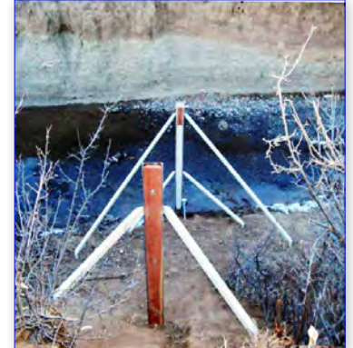
Back Side of Metal Brace for Lower Staff Gage
