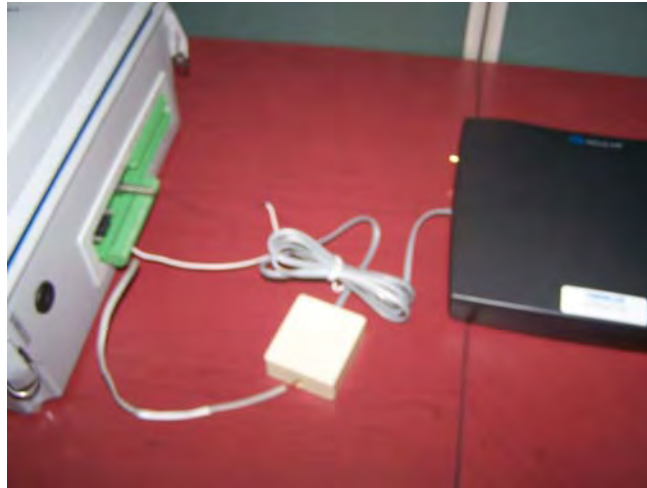
Figure 17. 8210 RJ11 adapter to FWT RJ11 jacks
