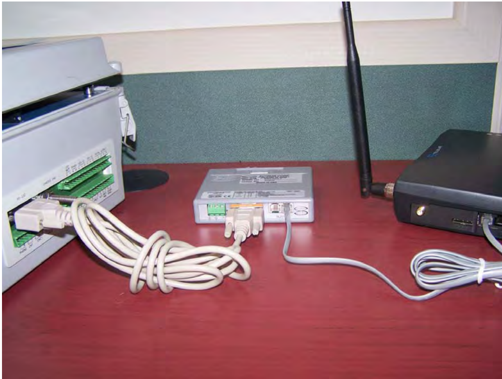
Figure 18. 8210 to speech modem to FWT connections
