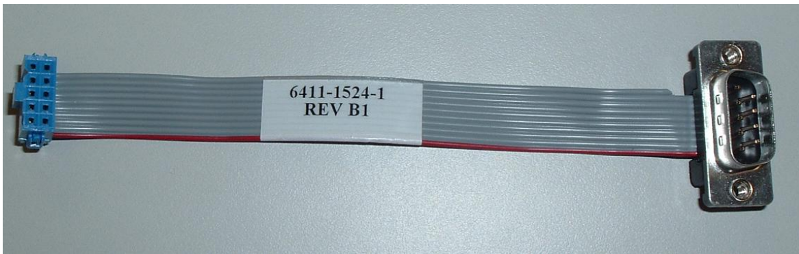
Figure 5 – Cable adapter to interface with a 9210/Xpert/8310
