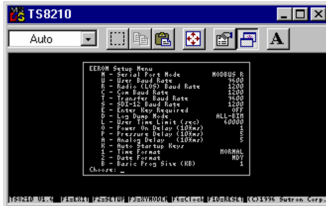
Figure 6 -- MODBUS RTU setting for serial port connections
