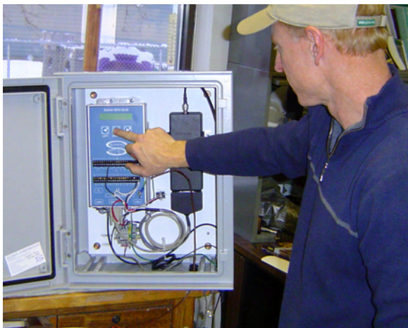
Sutron Hydro=Met Station in Antarctica featuring XLite Datalogger & Iridium Modem
